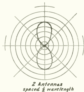
Four patterns of radiation depending on antenna spacing.
